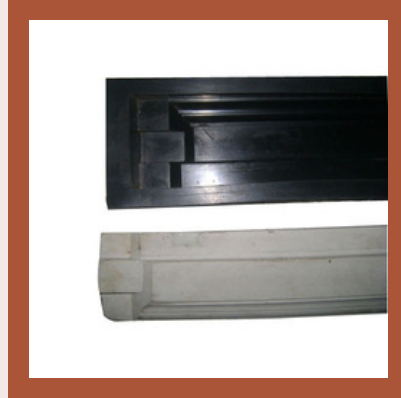
Reinforced Cement Concrete Rubber Mould
